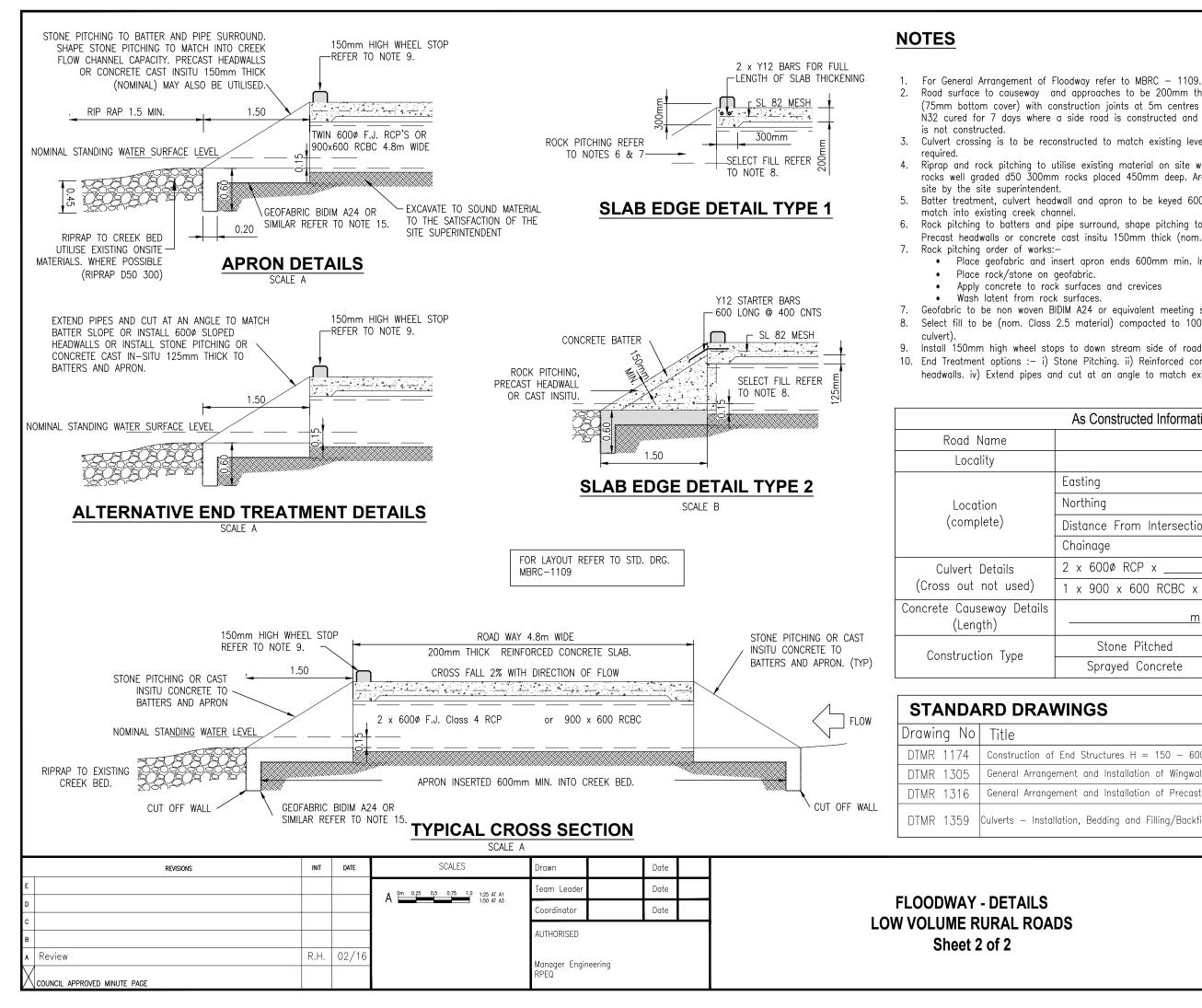
2. Road surface to causeway and approaches to be 200mm thick reinforced concrete with SL82 mesh (75mm bottom cover) with construction joints at 5m centres (max) or otherwise shown. Concrete to be N32 cured for 7 days where a side road is constructed and N50 cured for 12 hours where a side road
