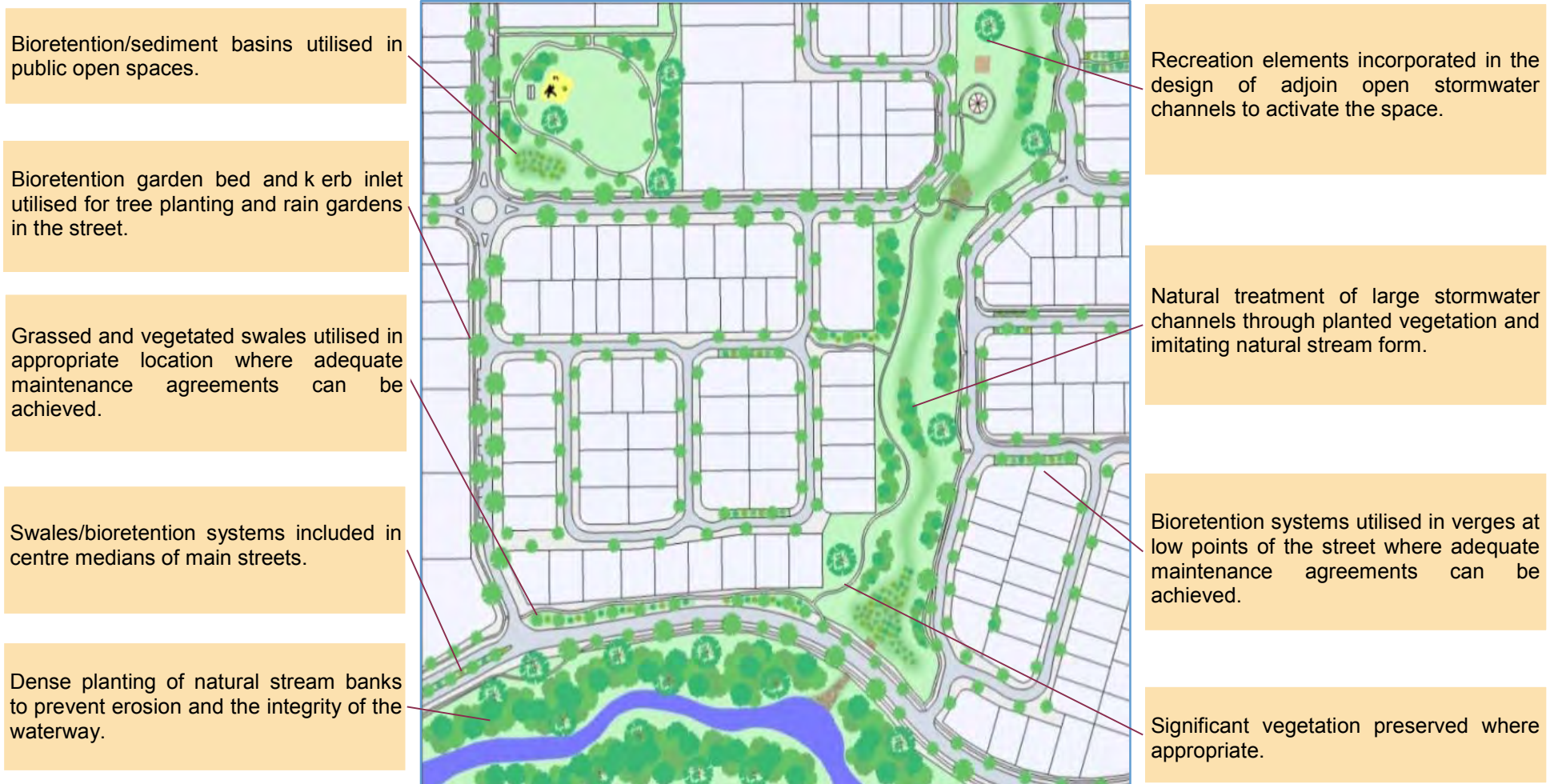
Figure 1.1: Indicative concept layout depicting possible locations for stormwater treatment in residential areas
