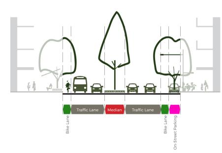
Figure 2: Typical Streetscape Cross Section for reference- Carriageway
