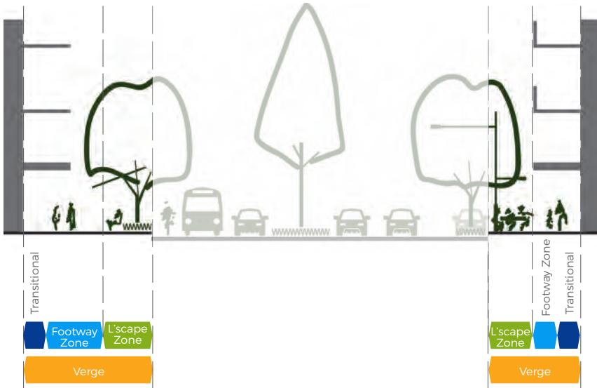
Figure 3: Streetscape Typical Cross Section for reference—Verge
