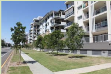
(Chermside) Basement car parks that protrude above natural ground level are setback behind screen landscaping, not just street trees as shown above.
