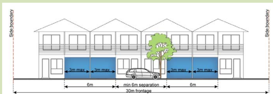
Example: Garage and carport openings
