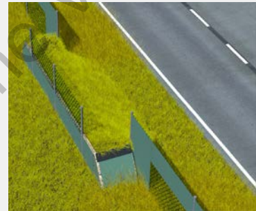
Concept design by Griffith University showing funnel fencing and escape areas for wildlife trapped between the road and exclusion fence.
