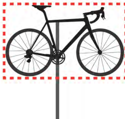
Continuous regular area using the outermost extremities around a three-dimensional advertising device.
