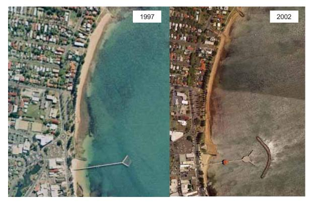
Figure 3-6 Accretion at Redcliffe Pier since construction of offshore breakwater
