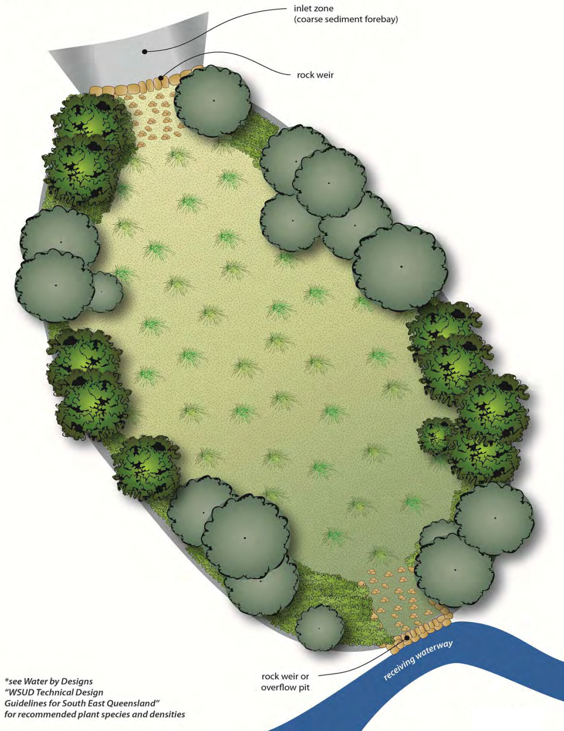
Typical Bioretention Basin Layout - Plan View
