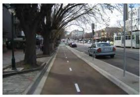
Figure 17 Raised kerbs provide separation from parked cars
