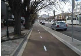
Figure 8 Example of one-way pair cycle infrastructure
