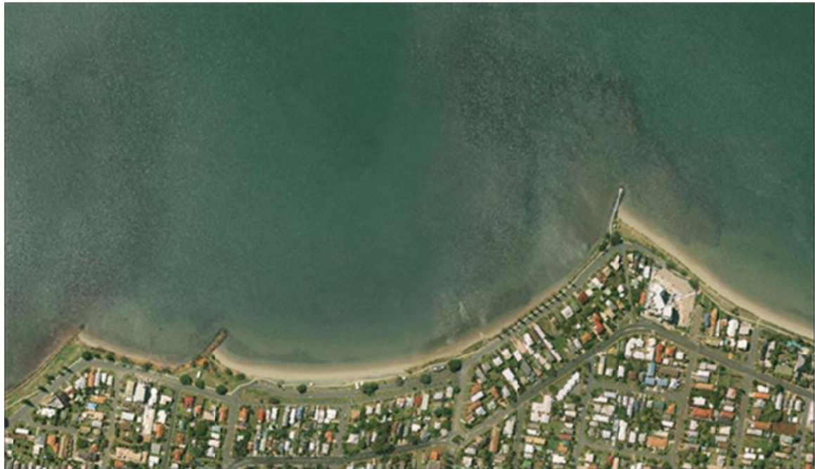
Figure 3-4 Groynes between Redcliffe and Scarborough
