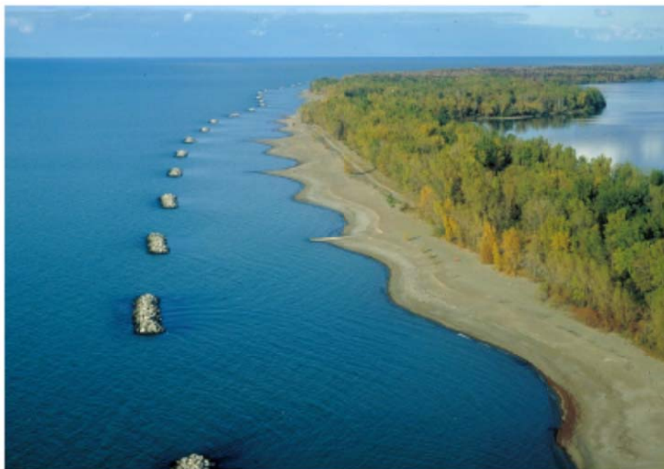
Figure 3-5 Offshore Breakwater Series and Salient Formation (U.S. Army Corps of Engineers, 2002)
