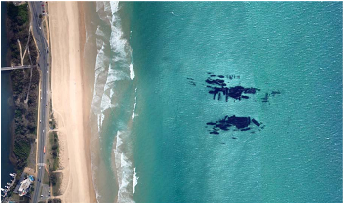
Figure 3-6 Geotextile Sand Container Artificial Reef at Narrowneck, Gold Coast (Source: NearMap, 2011)
