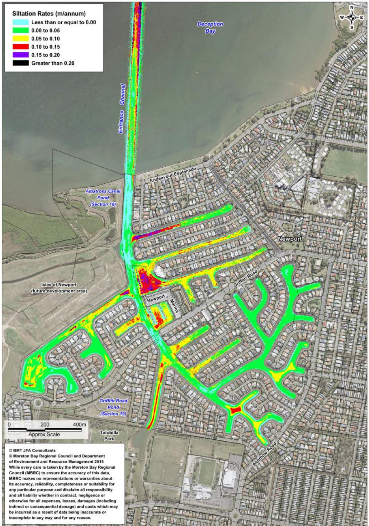
Figure 3-1 Canals - Estimated Siltation Rates 2009 to 2015
