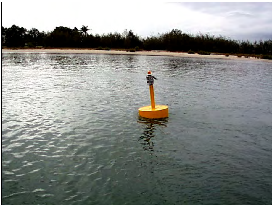
Figure 17. Deployed InterOcean S4 Current Meter (Banksia Beach).
