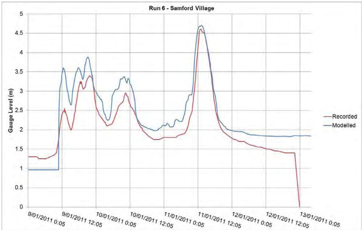
Figure 4-8 Flood Level Comparison at Samford Village
