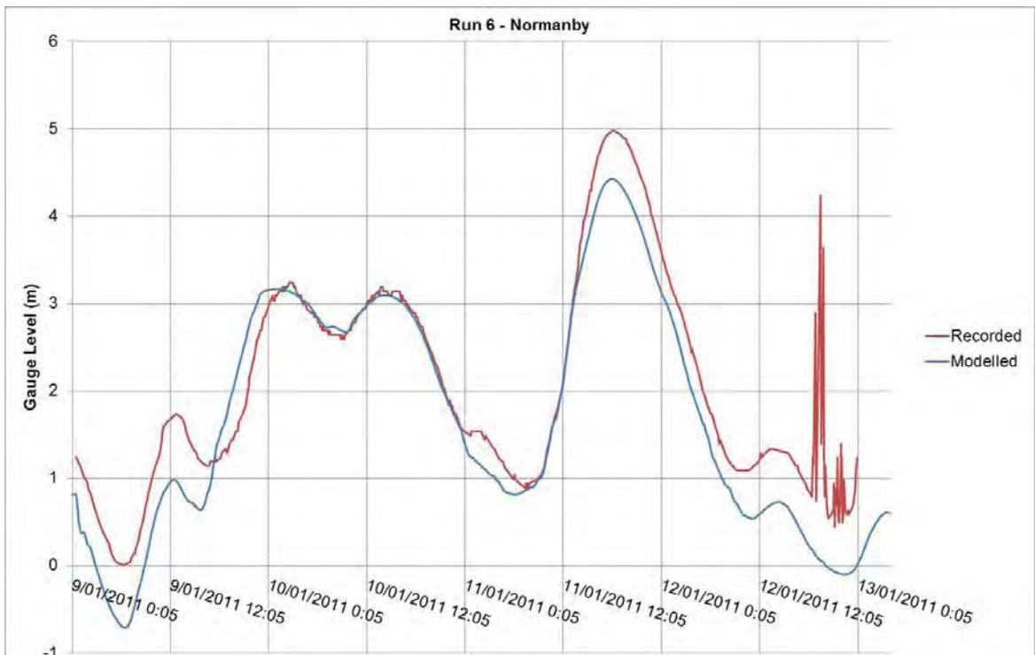
Figure 4-7 Flood Level Comparison at Normanby
