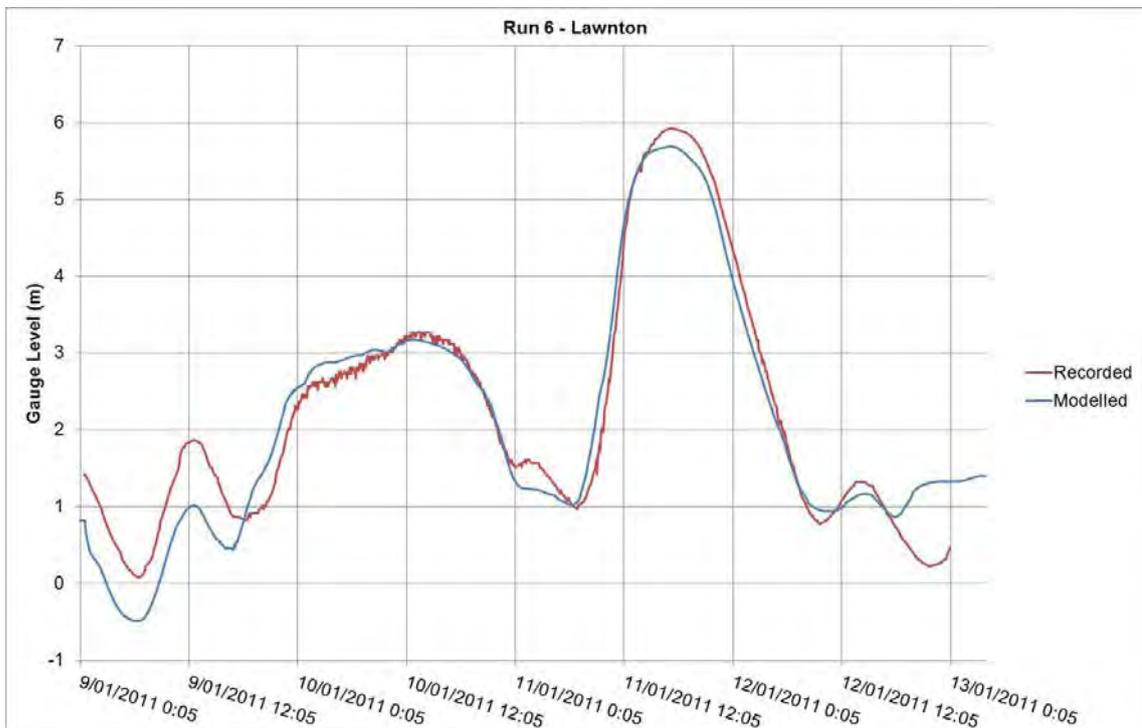
Figure 4-5 Flood Level Comparison at Lawnton
