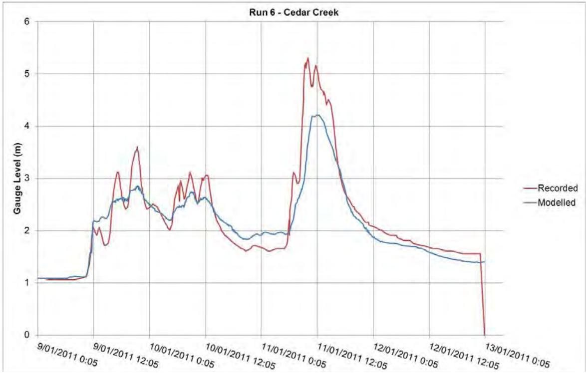
Figure 4-2 Flood Level Comparison at Cedar Creek
