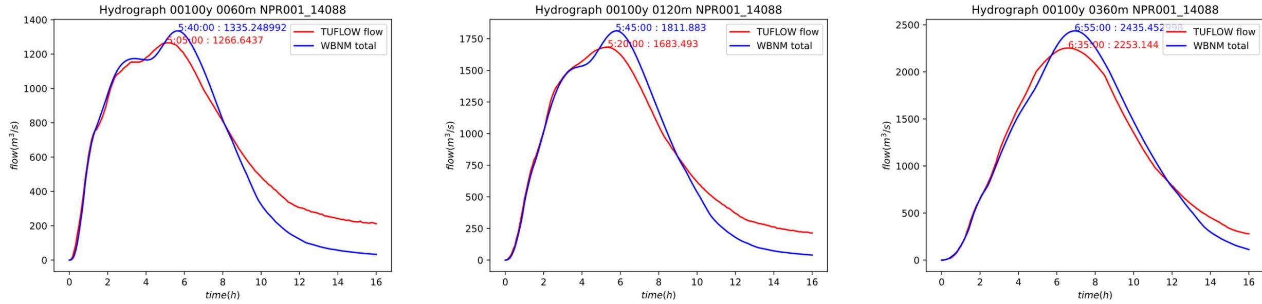
Figure 4.8 NPR001\_14088 for the 100-year ARI (left is 60-minute duration, middle is 120-minute duration, right is 360-minute duration)
