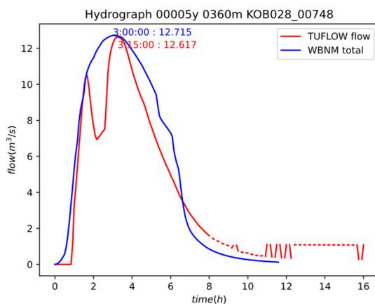
Figure 4.4 KOB028\_00748 double peak of the TUFLOW due to sub-catchment outlet not at the outlet of the storage
