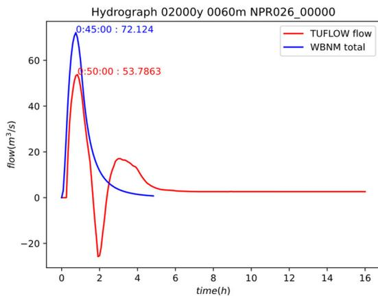
Figure 4.3 Backflow influence from the main creek in the TUFLOW results at NPR026\_00000
