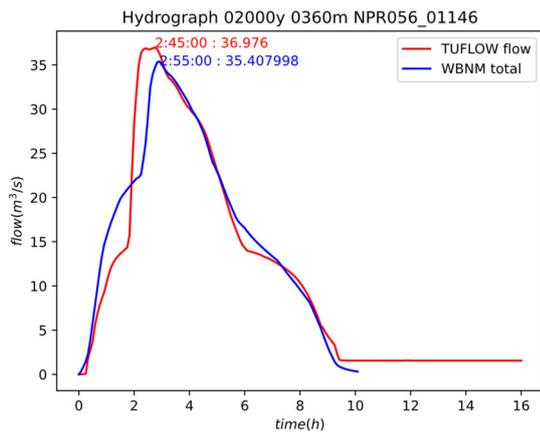
Figure 4.2 Overtopping at the upstream road creating a non-uniform shape in the TUFLOW results at NPR056\_01146
