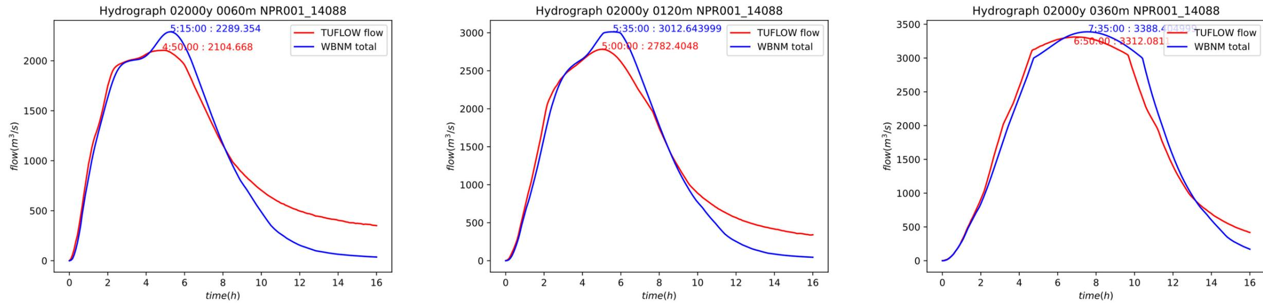
Figure 4.9 NPR001\_14088 for the 2000-year ARI (left is 60-minute duration, middle is 120-minute duration, right is 360-minute duration)
