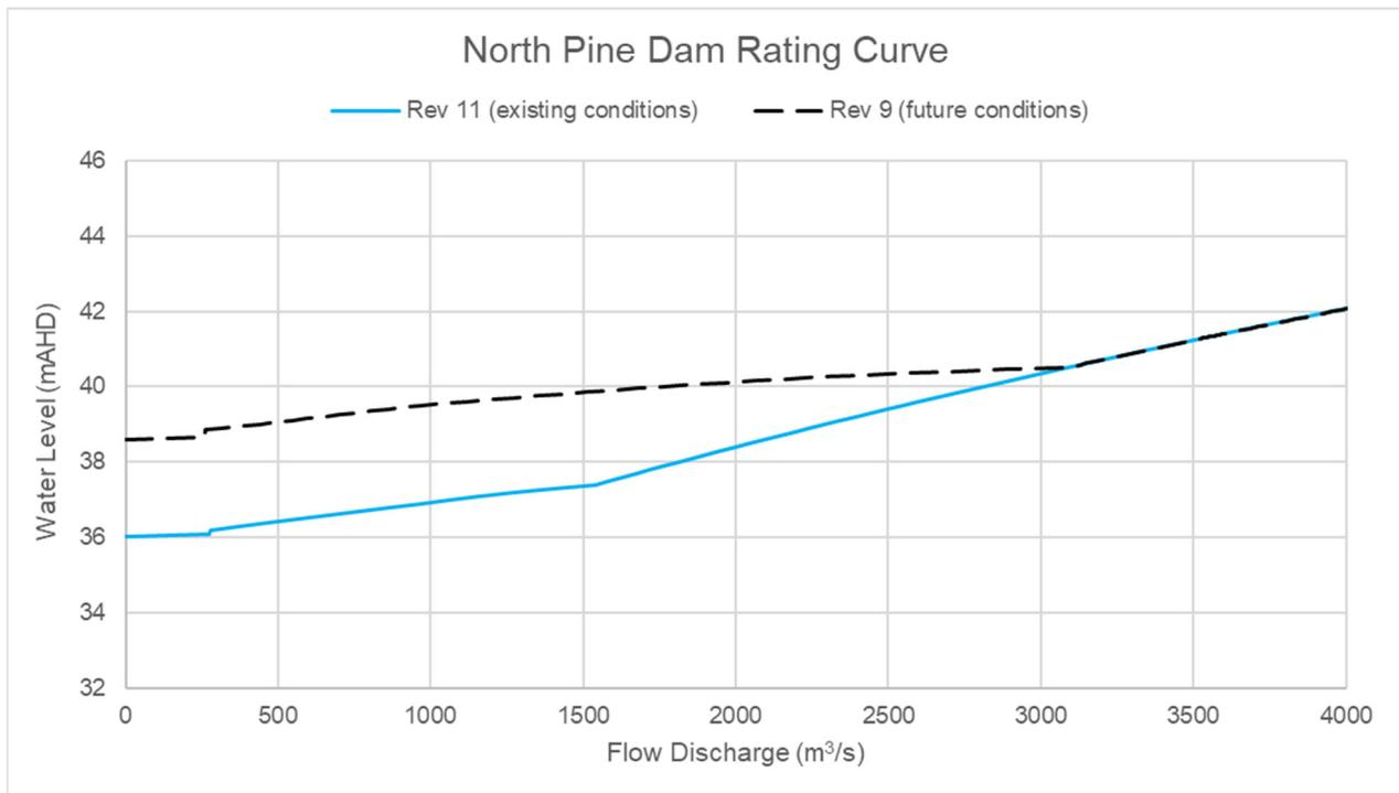
Figure 4.9 SEQWater Rating Curve at North Pine Dam
