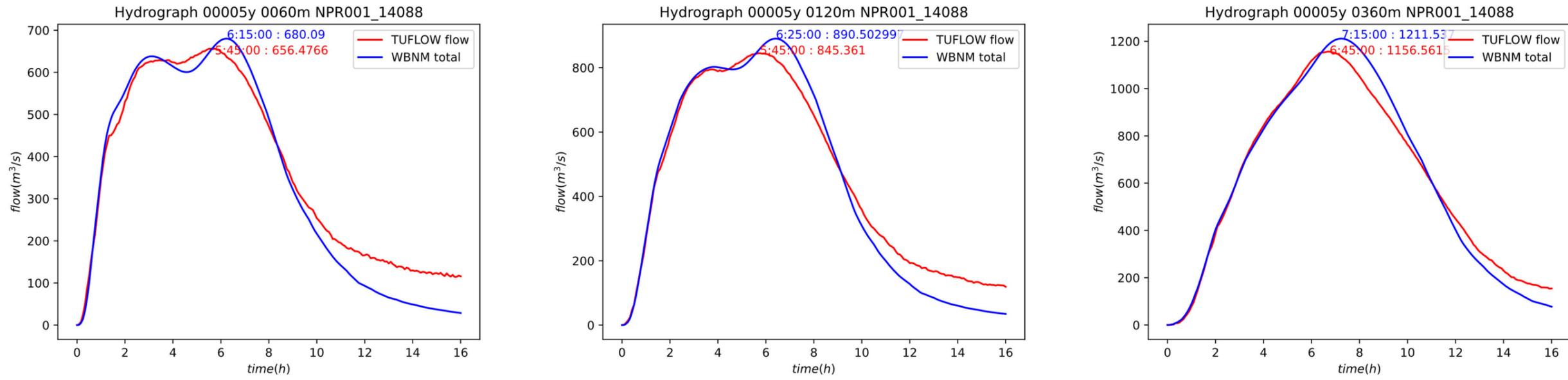
Figure 4.6 NPR001\_14088 for the 5-year ARI (left is 60-minute duration, middle is 120-minute duration, right is 360-minute duration)
