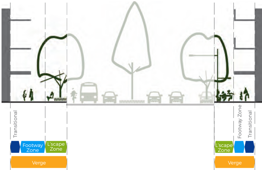
Figure 3: Streetscape Typical Cross Section for reference—Verge
