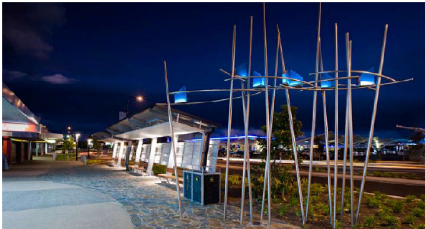
Use robust materials that do not deteriorate Make sure stainless steel is electropolished or use corten
