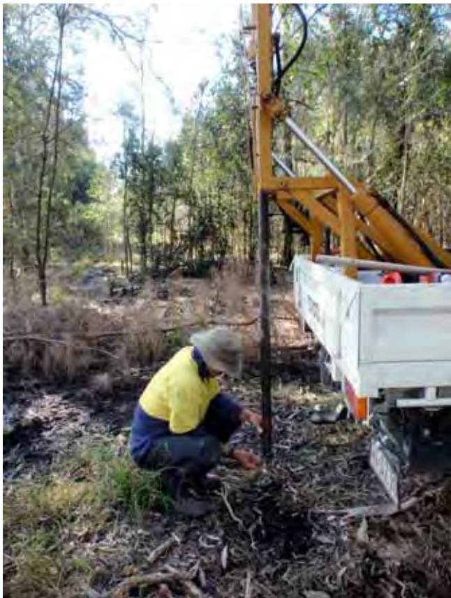
Photo 2: Hydraulic coring rig with steel tube
