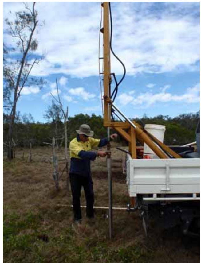
Photo 3: Hydraulic coring rig with tapered gouge auger
