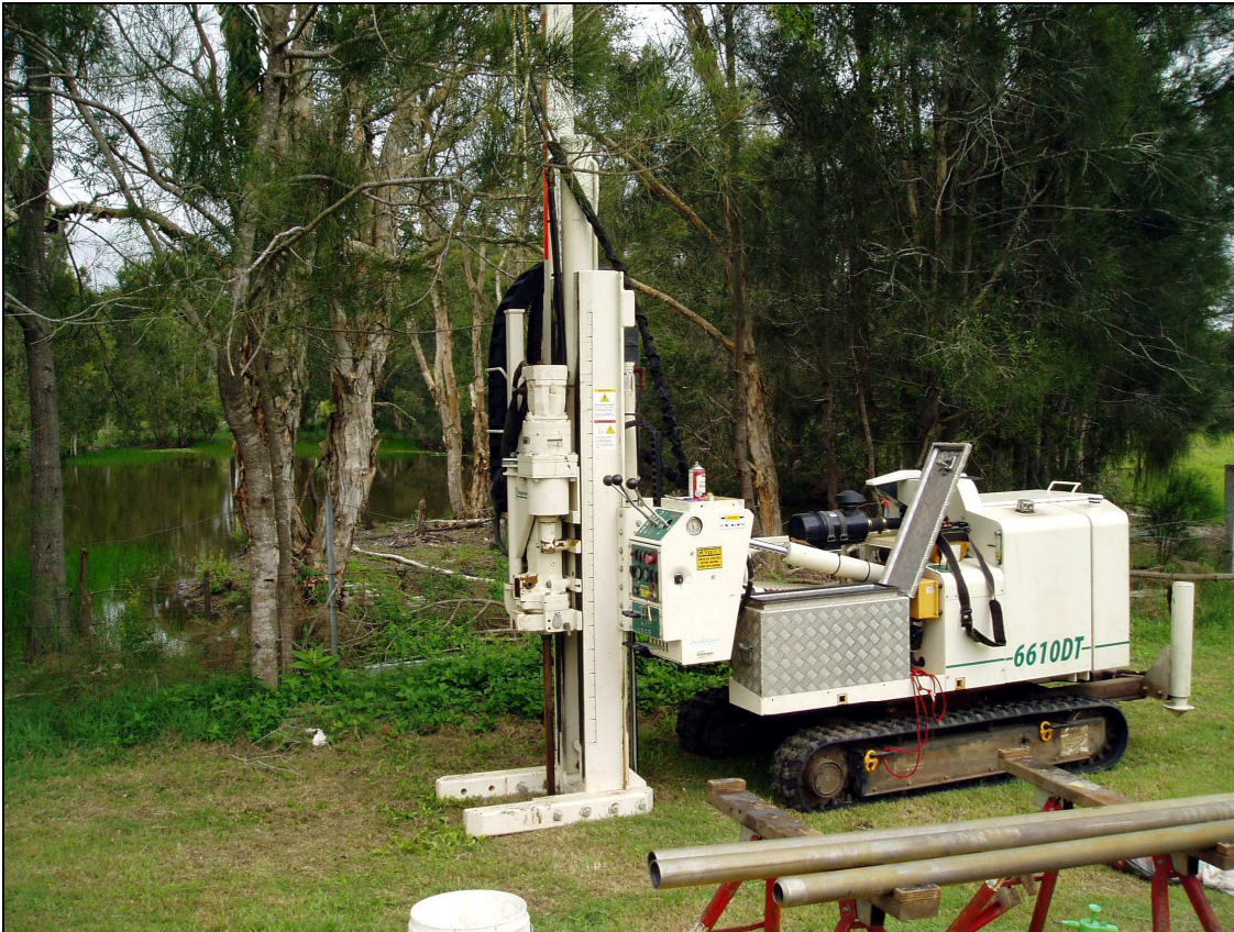
Plate 1. Geoprobe model 6610DT track-mounted coring machine
