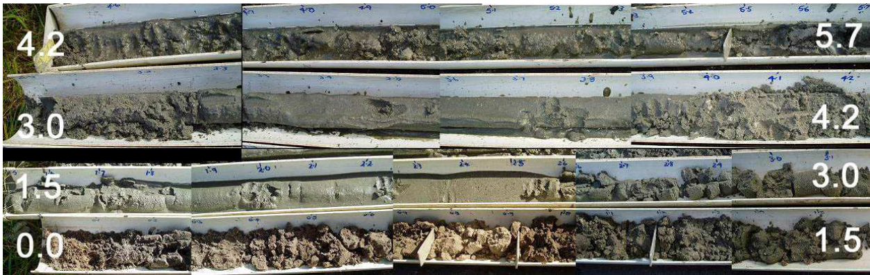
Plate 12. Soil profile CAB 60 showing PASS in lower layers
