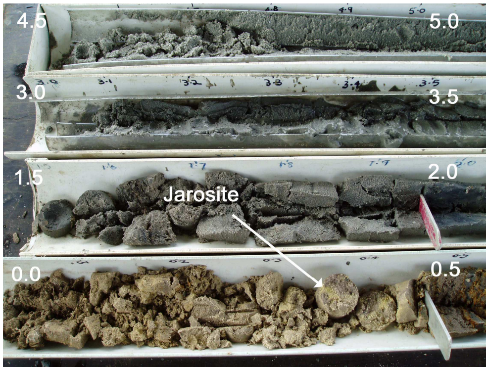
Plate 4. Yellow jarosite mottling in surface layers of CAB 96
