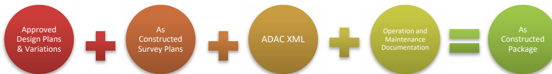
Figure 1 - MBRC As-Constructed Bundle Constituents
