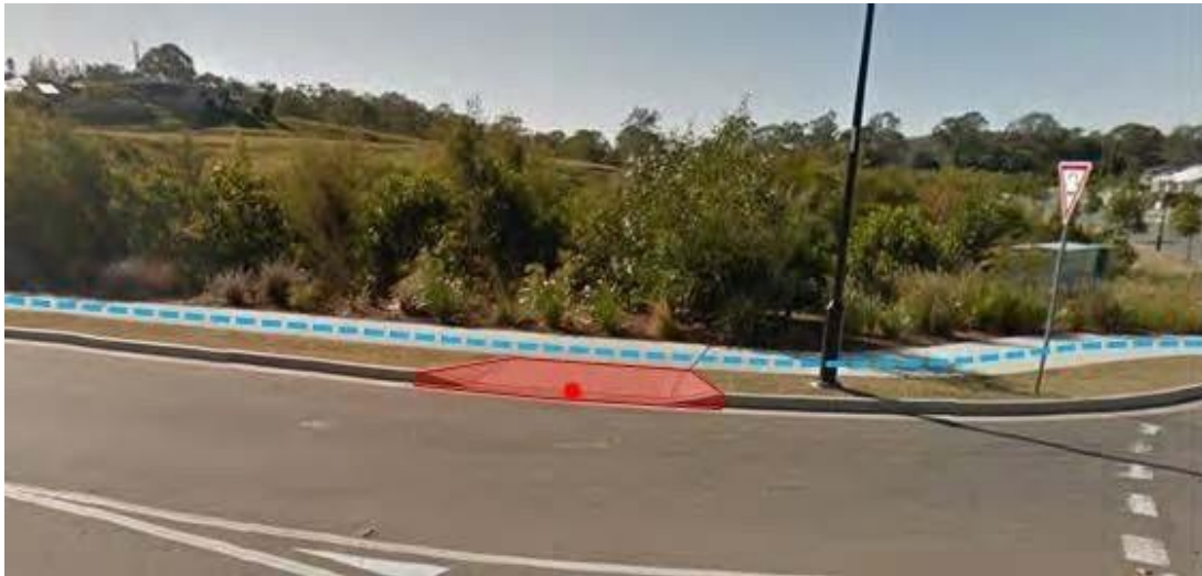
Figure 6: Pathway (blue) spatial representation with reference to a pram ramp (red polygon) and its spatial representation (red point) in the case where the pathway continues past the pram ramp.
