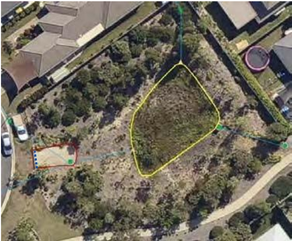
Figure 19: WSUD Area (yellow) and associated infrastructure including Vehicle Access (red) and Gate (blue dashed).
