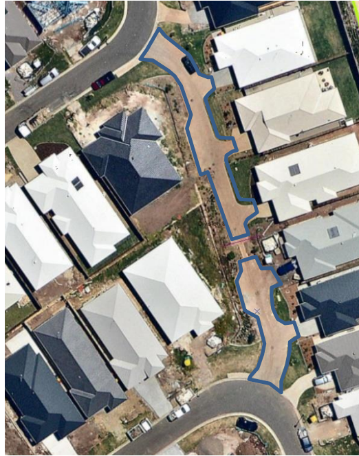
Figure 7: Access driveways to multiple properties (blue) or council assets should be captured as Pavement assets.
