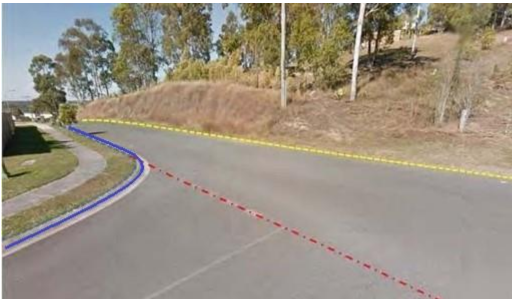
Figure 8: Spatial boundaries for pavement capture including where a kerb exists (blue), where no kerb exists (yellow) and where separate pavement areas a recorded for each road.
