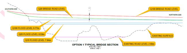
Figure 1 - Typical Bridge Section and Flood / Bridge Levels
