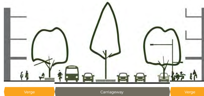
Figure 1: Streetscape Typical Cross Section for reference
