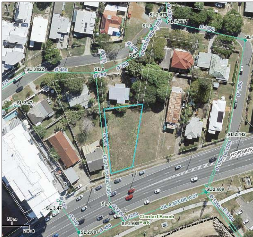
Figure 9: Existing Stormwater Infrastructure
