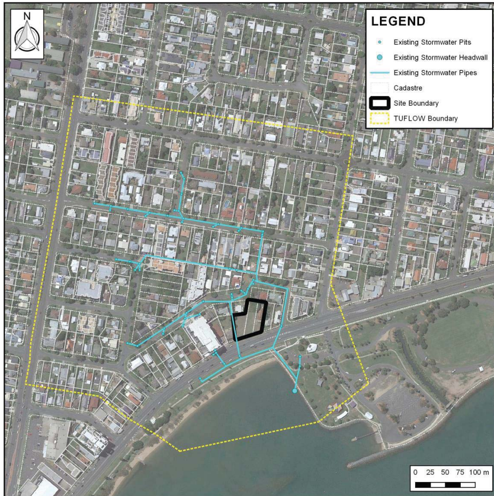
Figure 19: Pre-developed TUFLOW boundary and stormwater network
