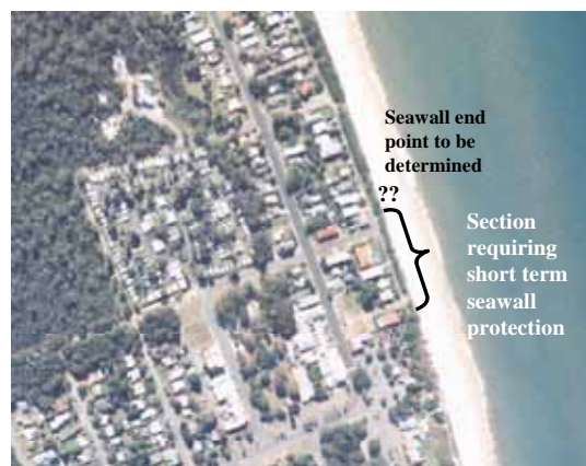
Figure 5-1 Section requiring short term seawall protection
