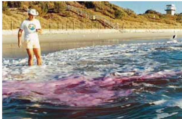
COPE Reading of Longshore Current at Woorim (approx 1985)
