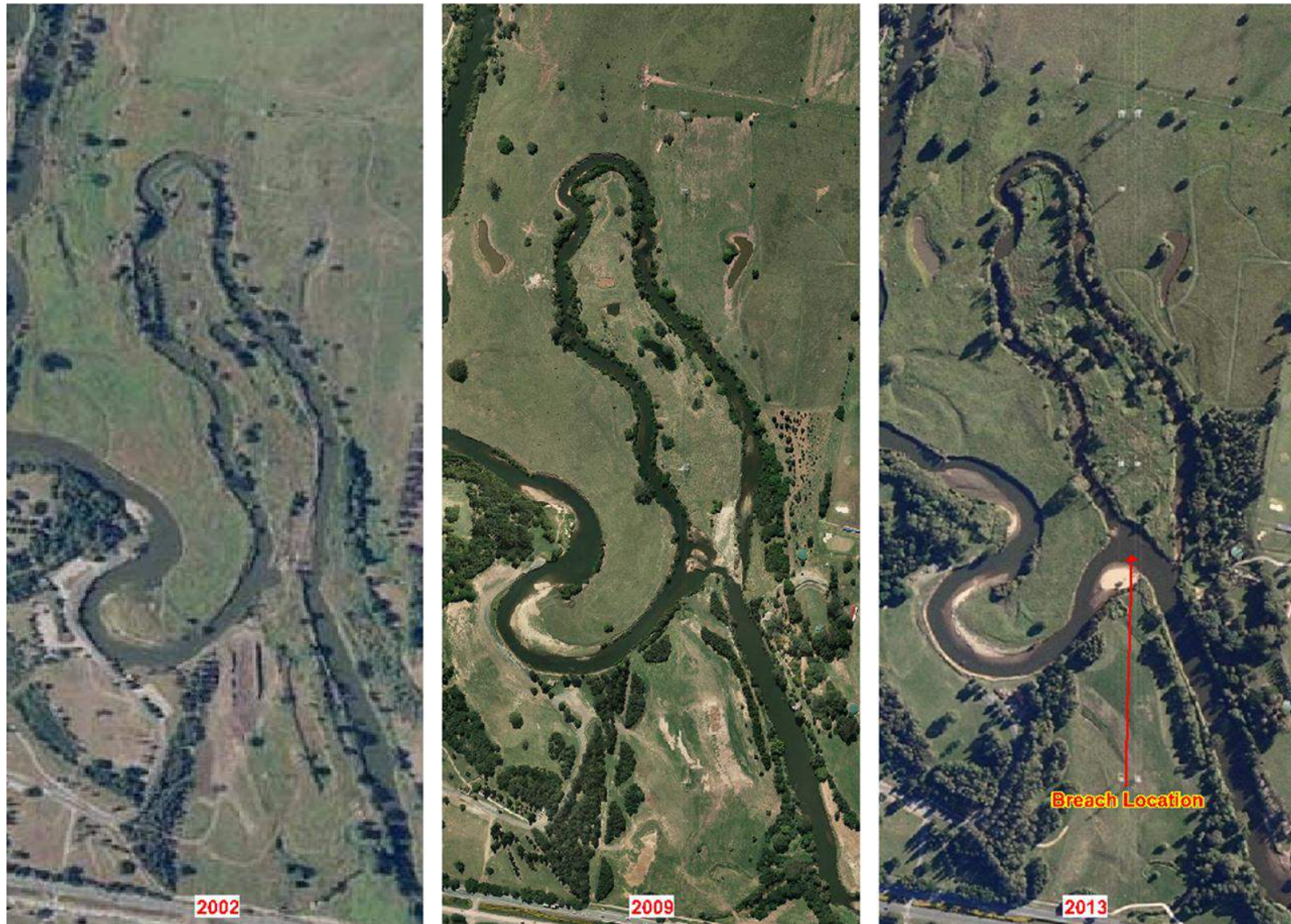
Figure 5-32 Breach at Pine Rivers Park
