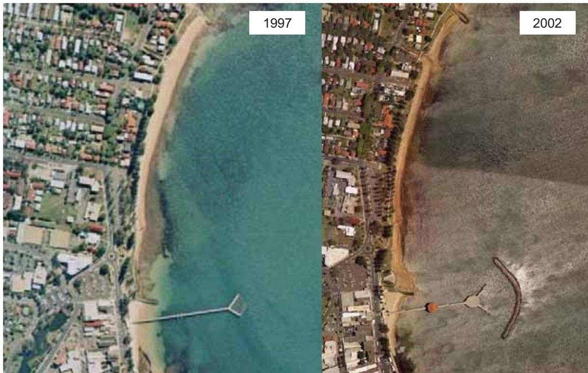
**Figure 3-6 Accretion at Redcliffe Pier since construction of offshore breakwater**
