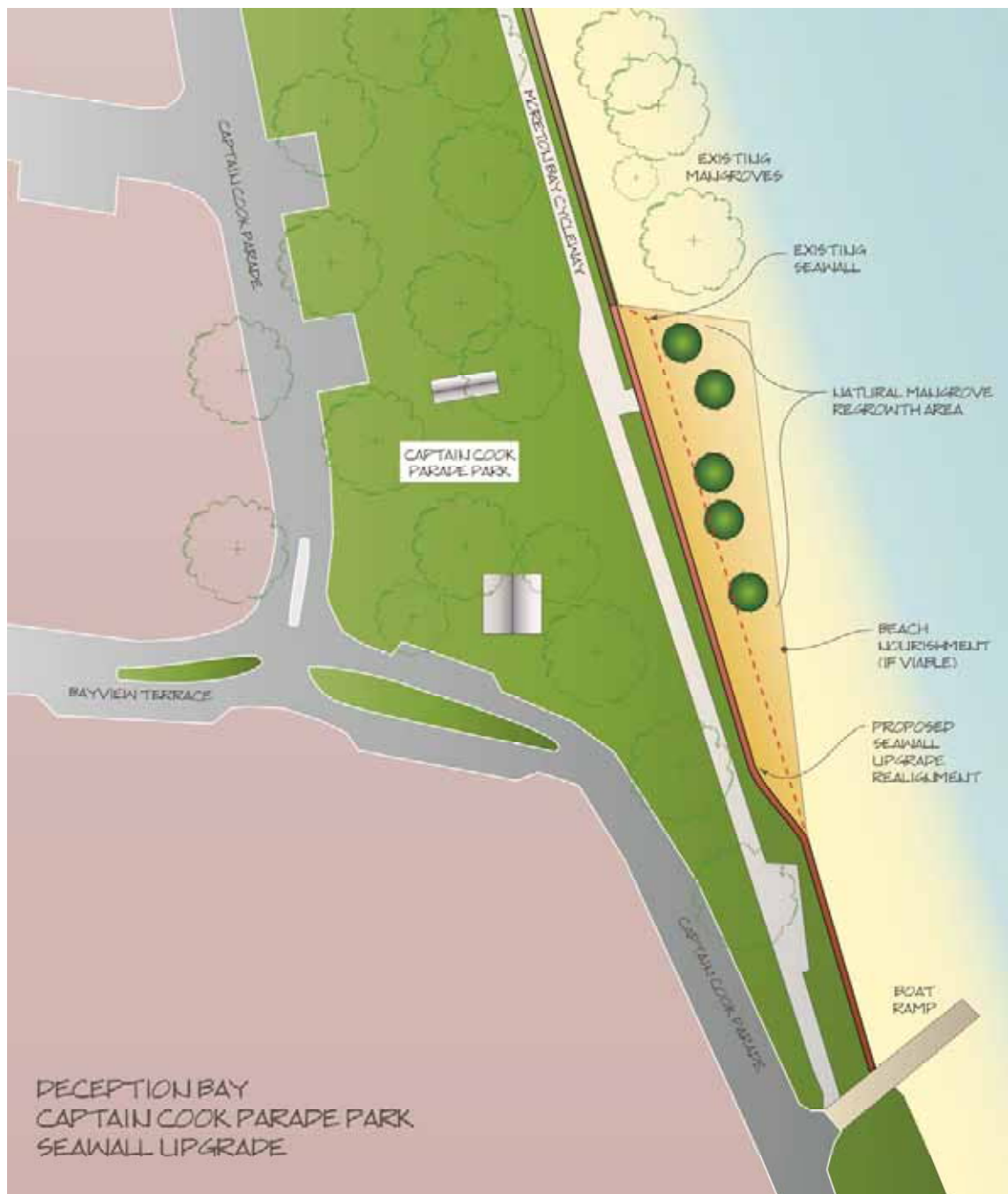
Figure 2-6 Captain Cook Parade Park Seawall Upgrade and Realignment and Mangrove Rehabilitation
