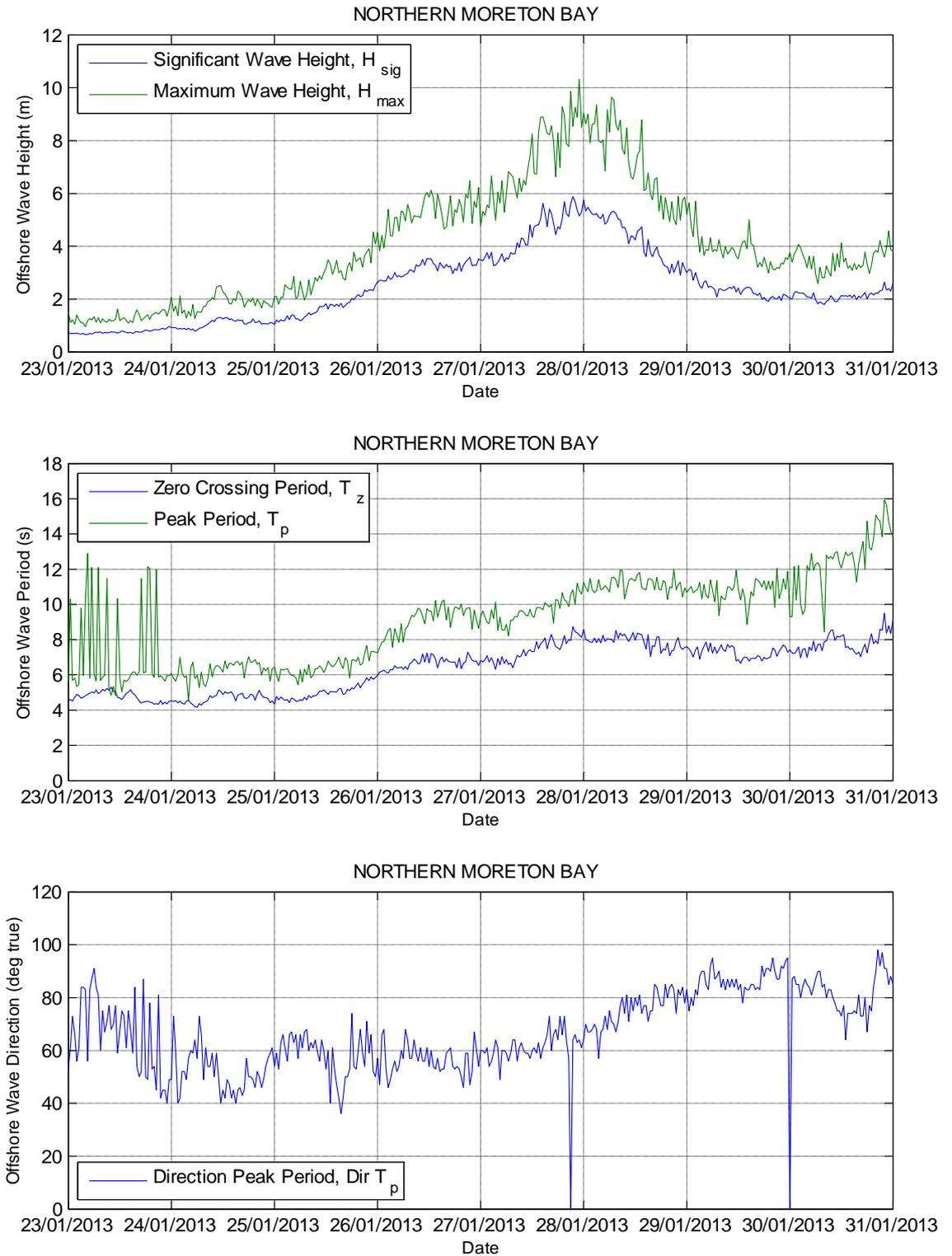
Figure 5-18 Recorded Wave Conditions Offshore from Bribie Island during ex-TC Oswald (data provided by DSITIA)
