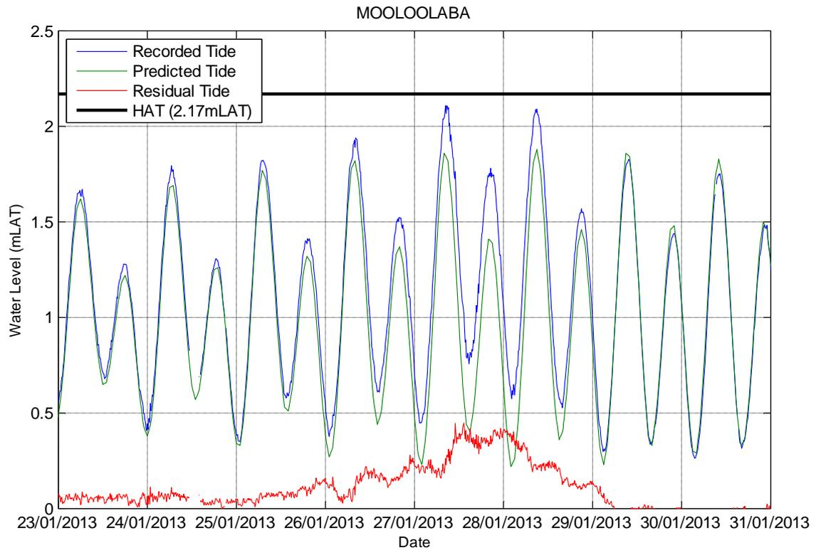
**Figure 5-17 Recorded, Predicted and Residual Tide at Mooloolaba Storm Tide Gauge during ex-TC Oswald (data provided by DSITIA)**
