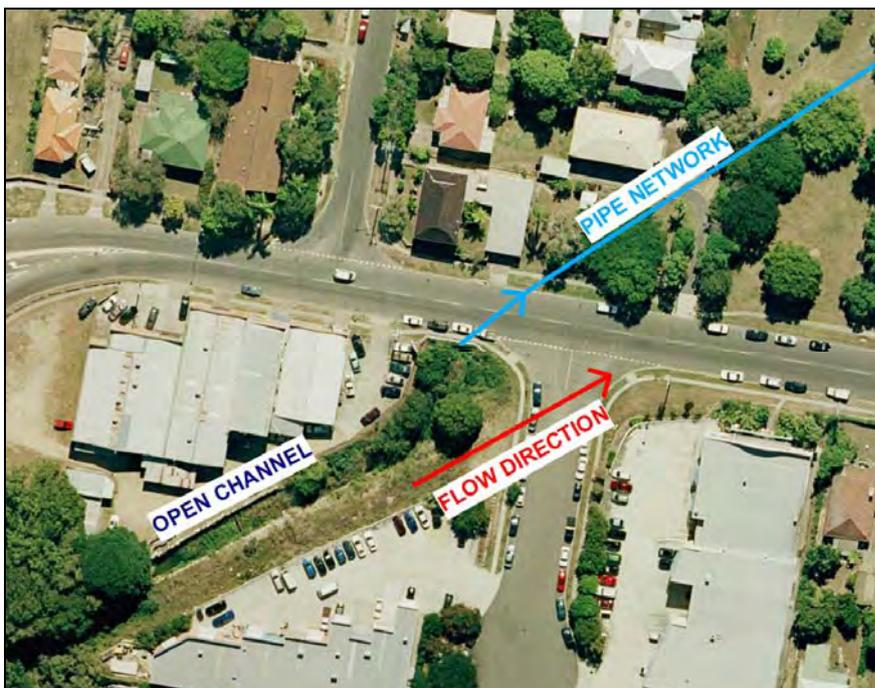
Figure 1 Example of Trunk Underground Drainage
