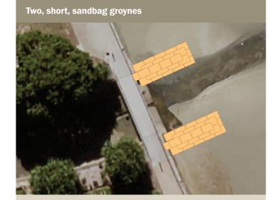
Approximate dimensions: Length 13 m x Width 5.4 m x Height 1.5m above ground, 1.5m below ground level
