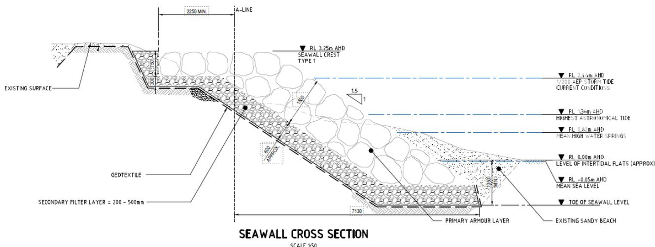
*A cross section of the standard seawall design included in the development approval application.*
