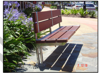
Facilities and furniture are to be installed on paved, concrete or other hard surfaces (Gympie Road, Strathpine)
