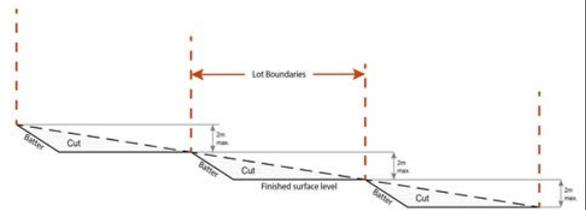
Note - Benching is to incorporate suitable measures to ensure stabilisation and prevent erosion.
