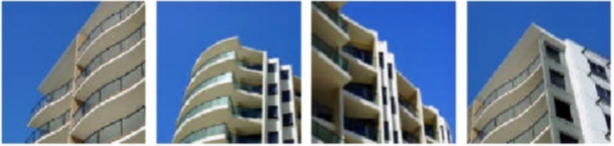
ii. balcony roofs, wall articulation expressed with different colours, curves in plan and section, and window awnings;
