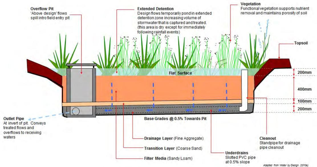
**Figure A-1 Conceptual Cross Section of Assumed Bioretention Properties**
