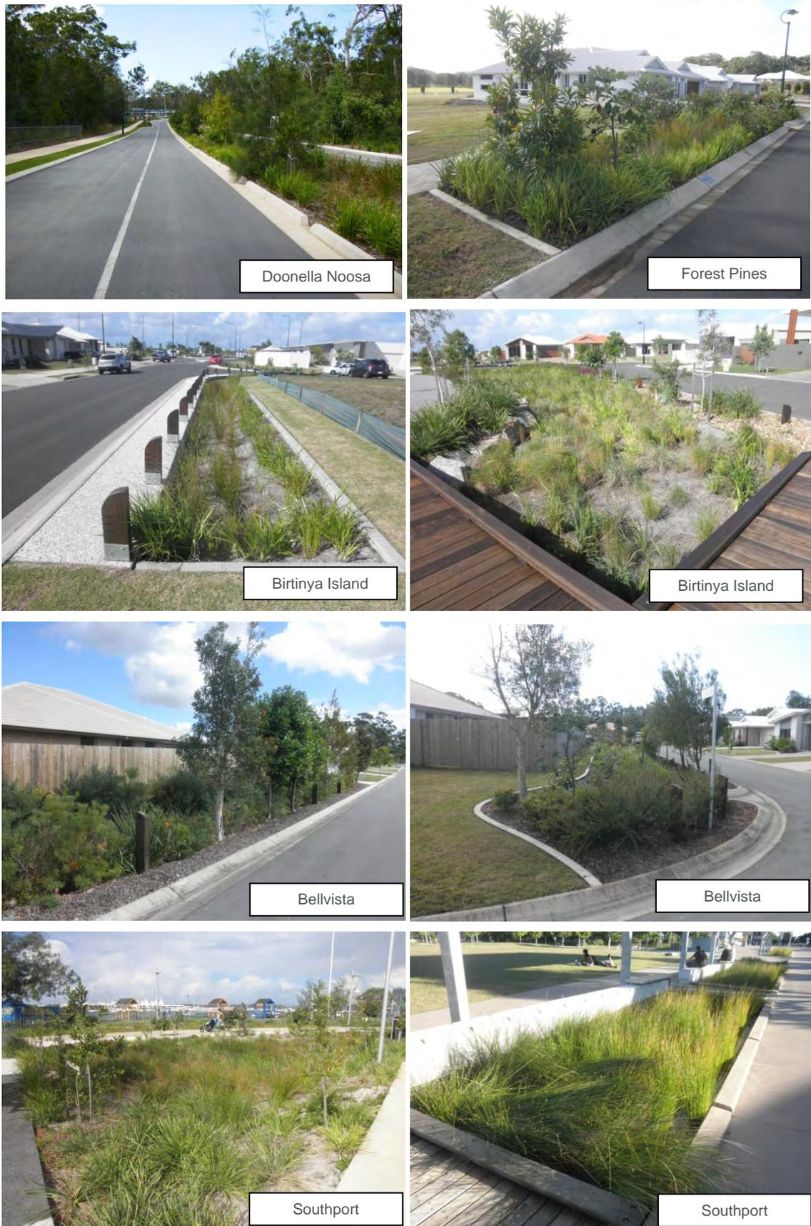
Figure 5-1 Examples of Streetscape Bioretention Systems in South East Queensland
