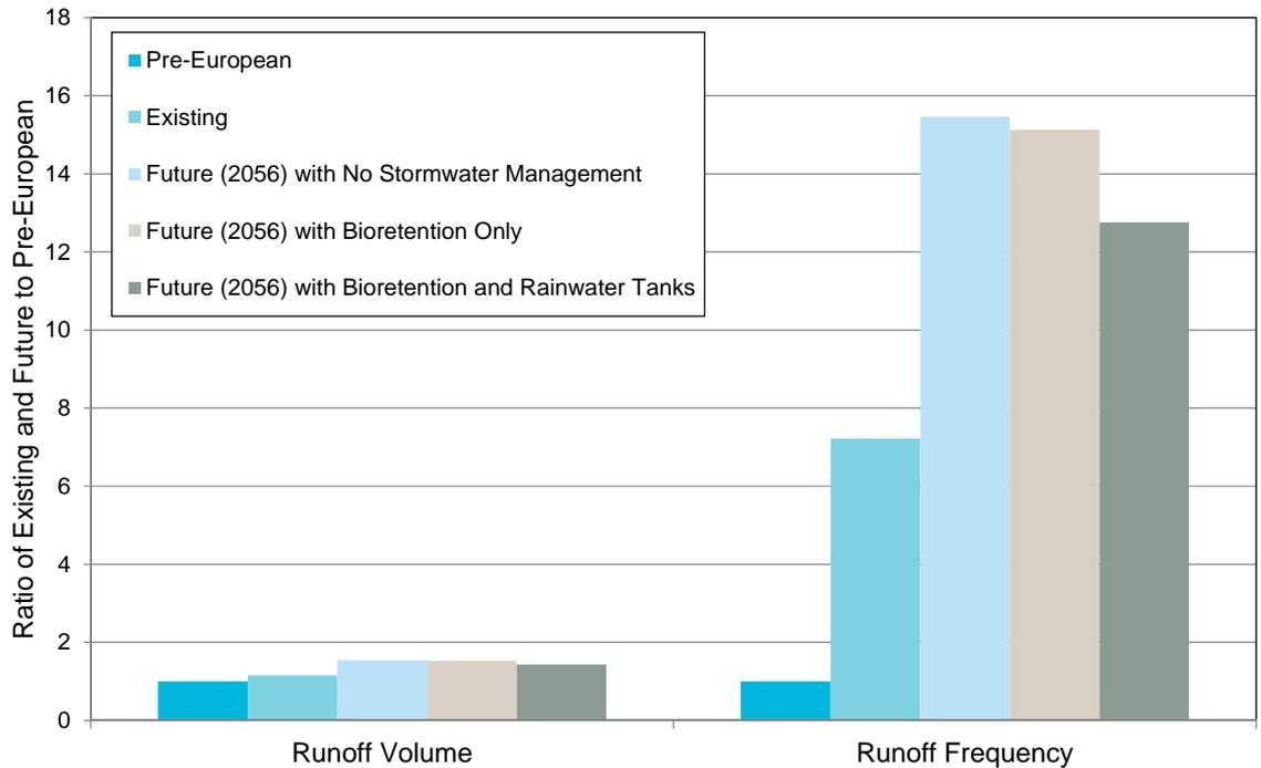
**Figure 6-4 Changes to Runoff Volume and Frequency as a Result of the Proposed Development and Impact of Including Rainwater Tanks**
