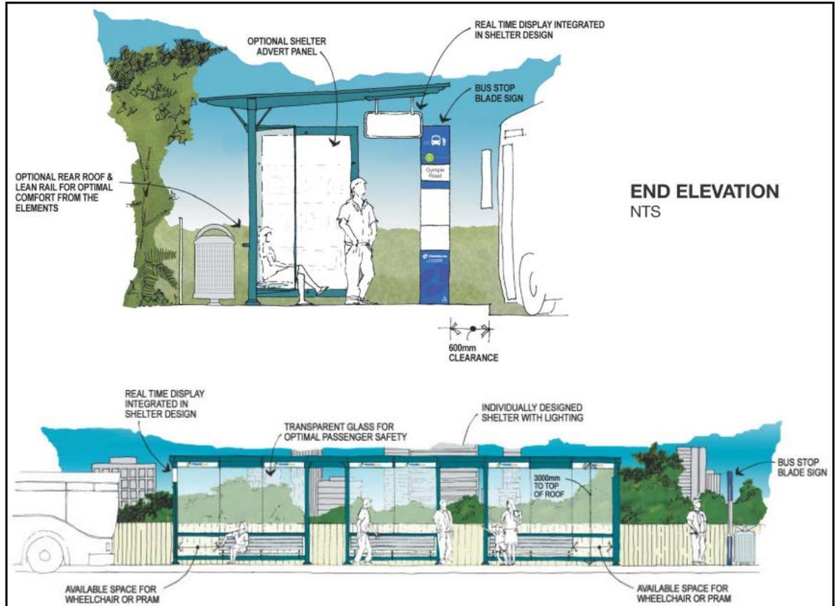
Figure 5.1 Example of a TransLink 'Signature' stop
