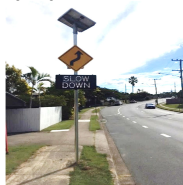
Figure 19 - Electronic Road Signage (Camelia Avenue, Everton Hills)
