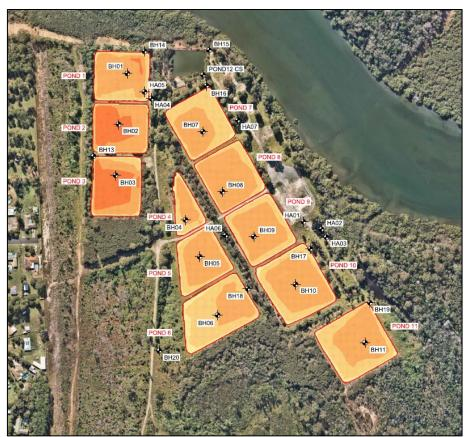
Figure 5 Pacific Harbour Maintenance Dredging project - Ningi dredged material placement site - 'pond' layout
