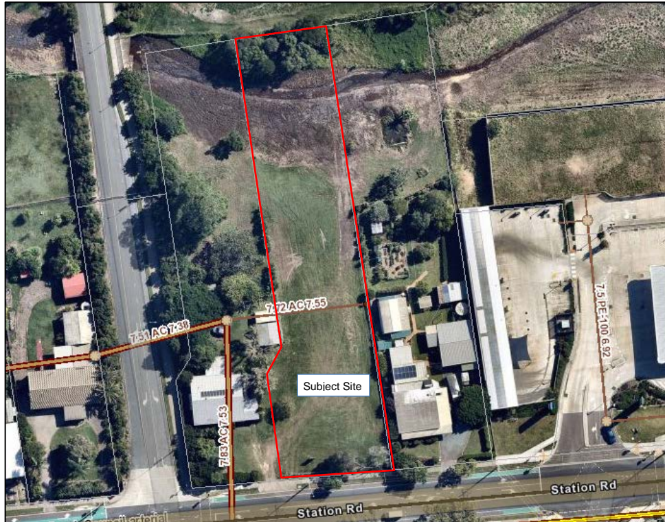
Figure 2 - Existing sewer infrastructure within the site
